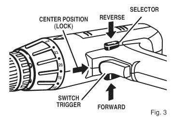
**CAUTION:** To prevent gear damage, always allow chuck to come to a complete stop before changing the direction of rotation.
